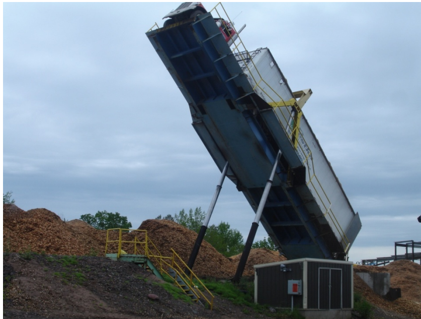
Figure B-1- Chip truck is tipped and unloaded at the facility close to the rail spur and piles of disposal ties-about half mile far from power plant (Photo by H. Pouryousef, Aug. 2011)
